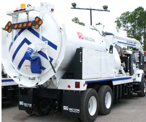
Vac-Con manufactures machines for sewer flushing and cleaning, as well as industrial vacuuming and hydro-excavation machines. The firm fabricates tons of steel plate, from 20 gauge to 2.5 in. thick.
