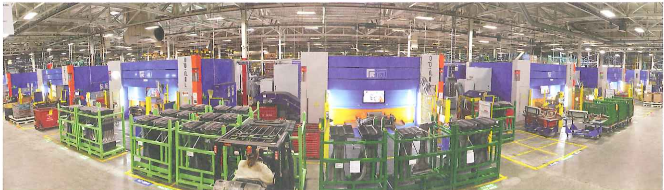
↑ Dozens of Rapido fiber are often installed in plants dedicated to hot stamped steel component cutting
