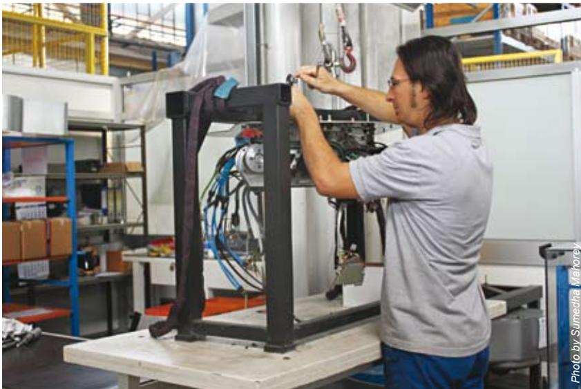
The laser head being assembled in a specialised assembly.
