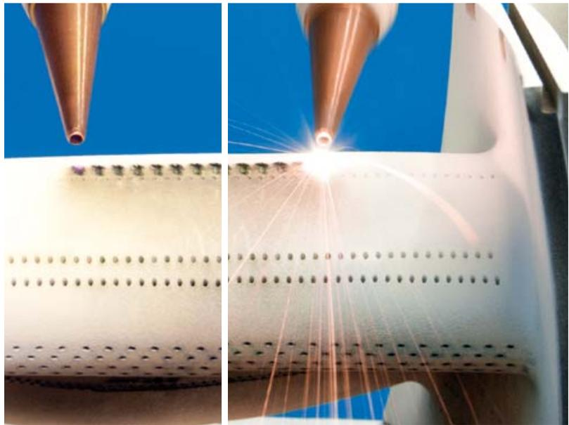
*Photos 3 & 4: Cooling hole design and manufacture hold the key to aerospace engine efficiency. Next generation engines call for denser cooling hole patterns and more complex holes. Only next generation laser systems can efficiently and economically produce these hole patterns.*
