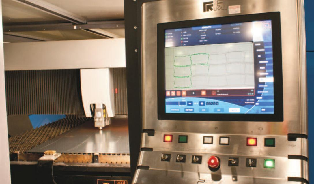
*ECCO installed its laser-cutting machine in August, 2011. The machine has a 120- by 60-in. worktable and a 6-in. z axis. Its unique architecture allows full accessibility to the working area from three sides.*
