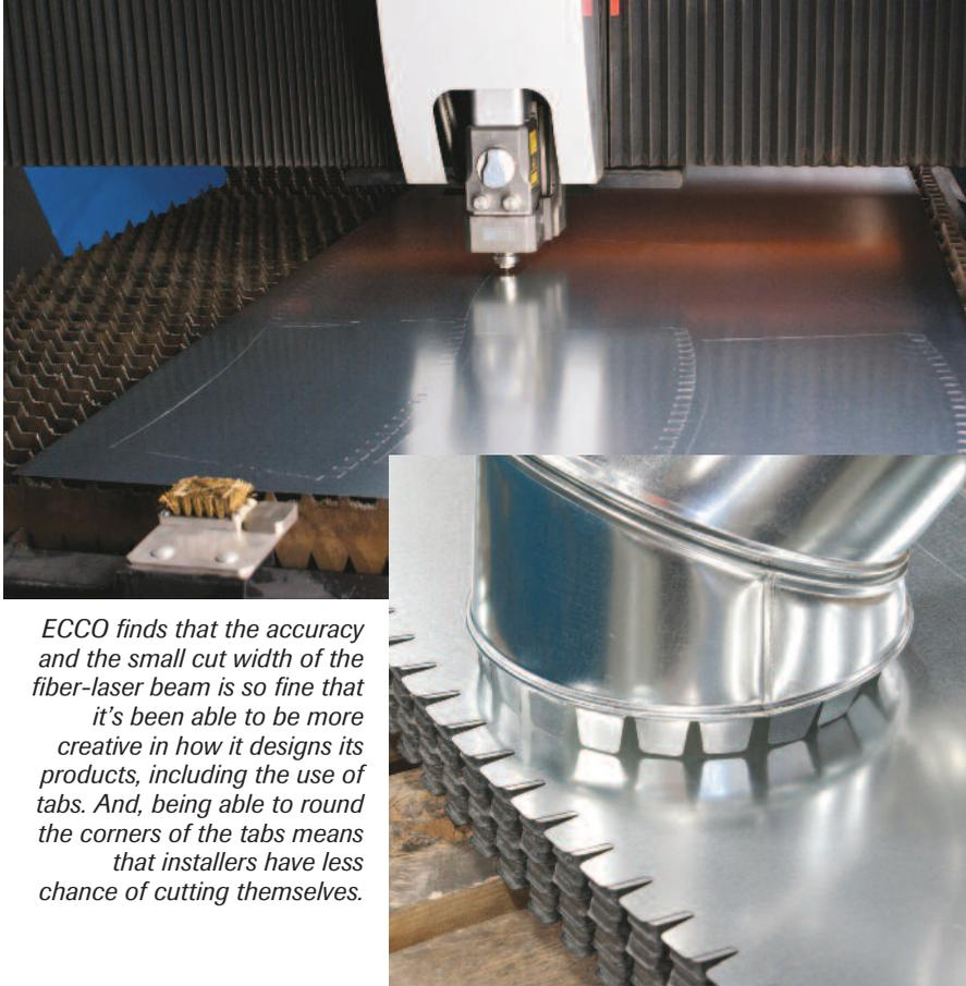
*ECCO finds that the accuracy and the small cut width of the fiber-laser beam is so fine that it's been able to be more creative in how it designs its products, including the use of tabs. And, being able to round the corners of the tabs means that installers have less chance of cutting themselves.*
