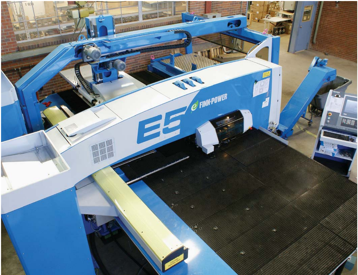
The E5 Compact Express adds unmanned operation through highly compact load/unload automation. With the E5, both the position and speed of the punch and die are programmable, which allows punching, nibbling, cutting, forming, marking, bending, and tapping in just a single setup.
