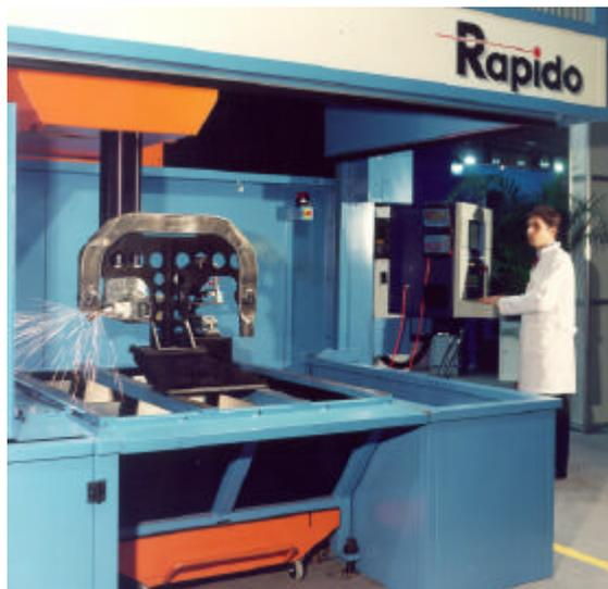
**RAPIDO**, the machine for the processing of medium and large three-dimensional components, is presented with the **Split Cabin**. "The laser solution" by PRIMA INDUSTRIE is shown in a production application: the fast cutting of automotive components. The machine work volume is divided into two parts to avoid idle times for loading and unloading.
