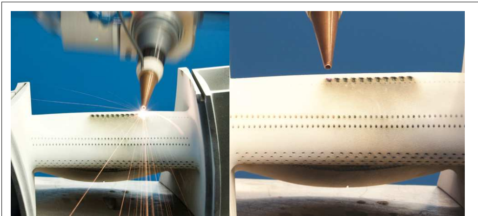
Caption Three And Four : Cooling hole design and manufacture hold the key to aerospace engine efficiency. Next generation engines call for denser cooling hole patterns and more complex holes. These cooling holes are very small, 0.5 - 0.75 mm diameter, at acute angles to the part surface. Only next generation laser systems can efficiently and economically produce these hole patterns.
