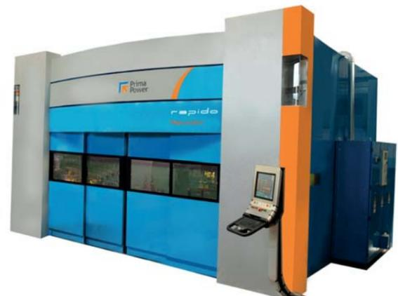
*The Rapido machine of Prima Power for three-dimensional laser cutting*
