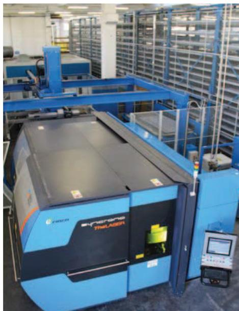
The Sincrono Fiber installed at Rizzato is connected to the automated and synchronized Night Train Material Management System (MMS), which allows a 24-hours-a-day operation for processing continuity.
