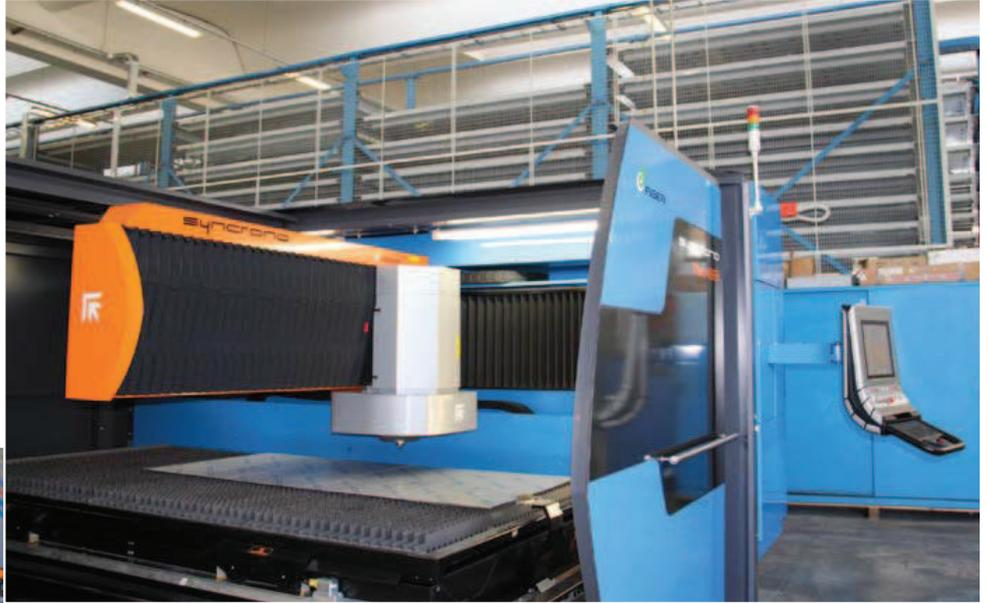
A key feature of Syncrono is the adoption of a parallel kinematics structure with the cutting head capable of reaching 6g accelerations and a numerical control which allows it to reach very high speeds even with very complicated trajectories.
