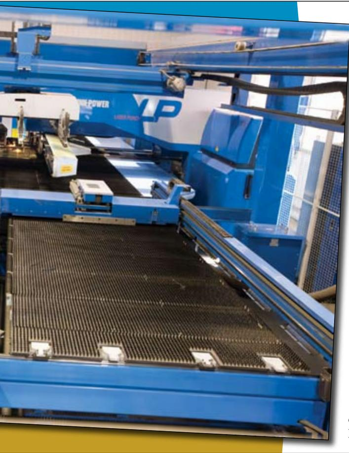
advantage is that all dies are at the same height and there are more high forming dies in the turret, reducing risk of material damage and increasing machine uptime.
