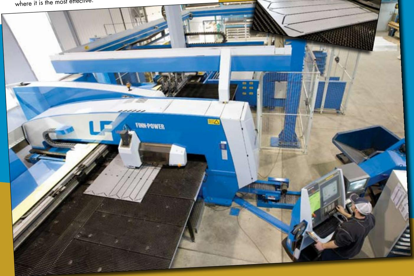
diffusion-cooled CO<sub>2</sub> SLAB laser that is integrated into the LP6. The focal length lens can be changed in seconds using a cartridge technique, and no tools are required. The cartridges are available in 5 and 7.5 in.
