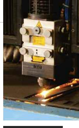
The Maximo is a large cutting system based on the Platino 2-D laser machine. It travels on rails over a fixed working table, processing sheets of any length.
