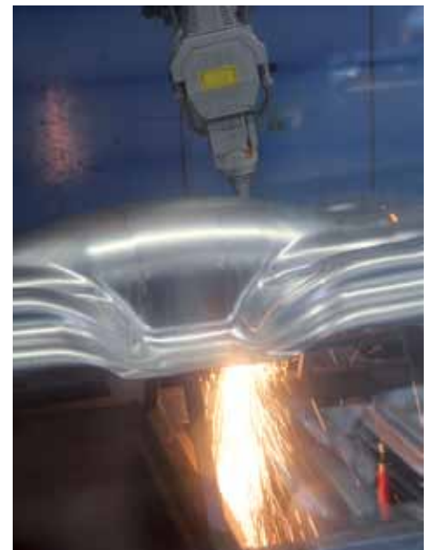
Nitrogen cutting of aluminum leaves the piece clean, and this is extremely important since the vehicle is not painted.
