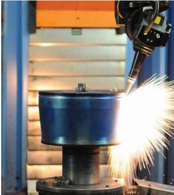
With nine Laserdyne multi-axis laser systems in-house, Ace Precision is equipped and experienced at the most complex projects requiring laser processing. As pictured, these include drilling effusion cooling holes in very dense patterns at shallow angles holding hole diameter tolerances of less than 0.002 inch.
