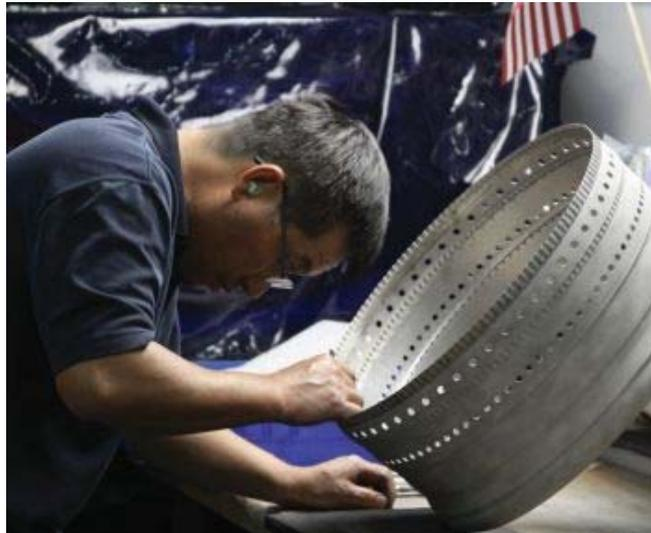
Ace Precision manufactures engine components for the commercial and defense industries. A laser-processed engine component is pictured being visually inspected. Ace Precision has experience with many engine designs including military platforms for Apache and Chinook helicopters, Abrams M1 Battle Tanks and B2, F18, F22 and F35 aircraft.
