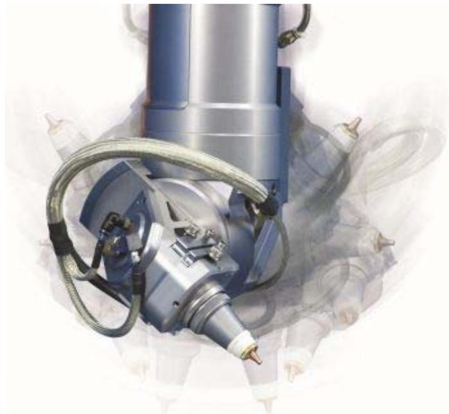
The motion required for multi-axis laser is very complex. Laserdyne's AFC features makes trepanning, percussion drilling and drilling on the fly fast, precise and with high quality results. The photo shows this complex motion simulation made possible by dual processors.
