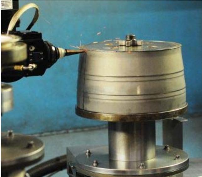
One of five Co2 laser systems ranging from 1700 to 4000 Watts used for cutting, trimming, welding, and hole drilling.
