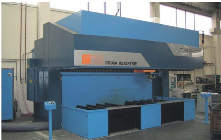
The jewel of the Impea line is Rapido, the machine for 3D laser cutting by Prima Industrie.
