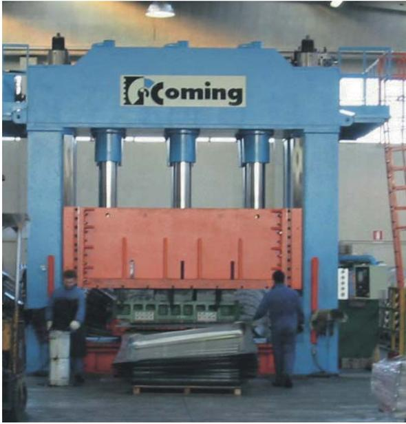
The Impea productive department uses mechanical and hydraulic presses that initially "deform" the sheet of metal plate to then pass it to the cutting and welding processes
