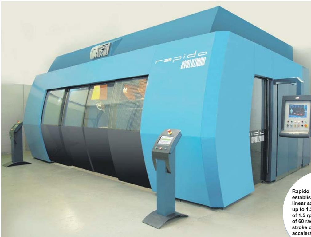
Rapido Evoluzione has established new frontiers: linear axes with acceleration up to 1.2 g, direct drive head of 1.5 rps and acceleration of 60 rad/s<sup>2</sup>, new C axis with stroke of  $\pm 10$  mm and record acceleration of 4 g
