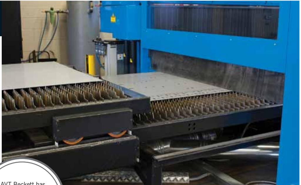
AVT Beckett has increased cutting speeds and improved cut quality with the new Platino 2D laser cutting machine.
