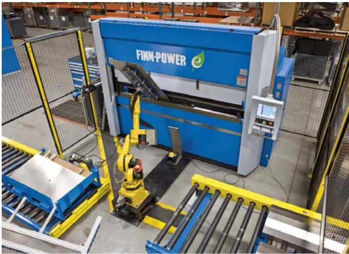
**Figure 5** As enclosures have become a bigger part of its business, Orion has found that its automation investments, such as its robotic press brakes, have helped it keep up with the growth.
