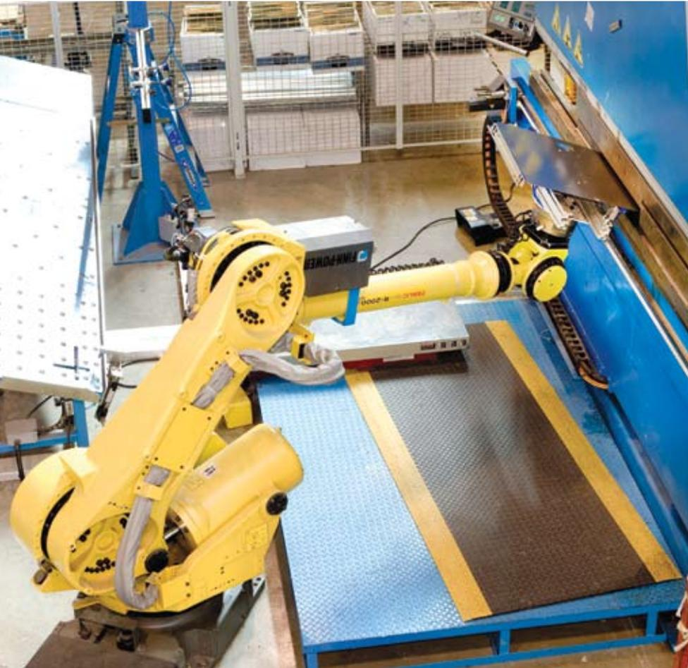
**Day-Brite had a series of parts that required two operators to form a complete part. With the robotic press brake from Finn-Power, the company reports a labor savings of 40 percent of each part bent.**
