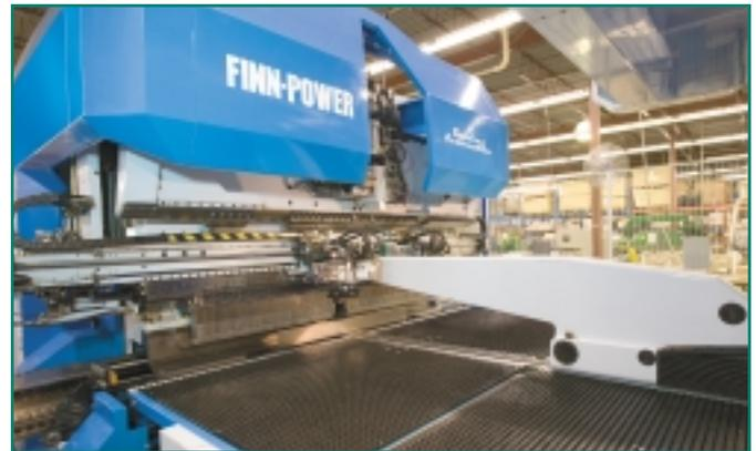
*The Finn-Power Express Bender enhances productivity by bending extremely high-quality parts in an unmanned environment in any quantities. Sheet sizes and part complexity can vary greatly with a machine capacity up to 11 gauge.*
