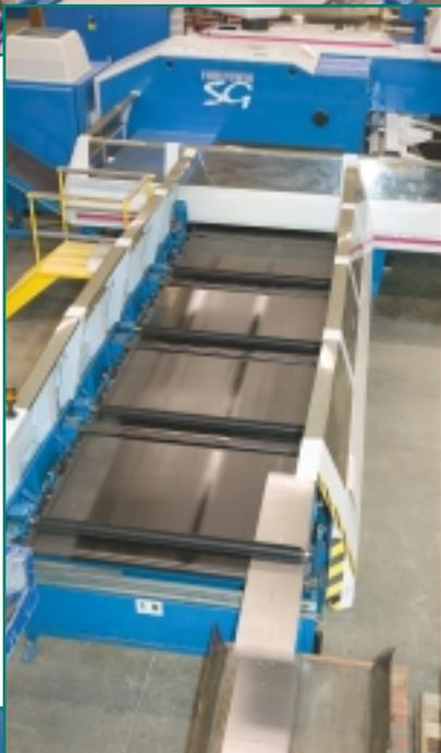
*With the Shear Genius concept, the objective is to provide a machine capable of transforming a full-size sheet into finished parts. These parts can be moved to the final production stages for immediate integration directly into the final product assembly.*
