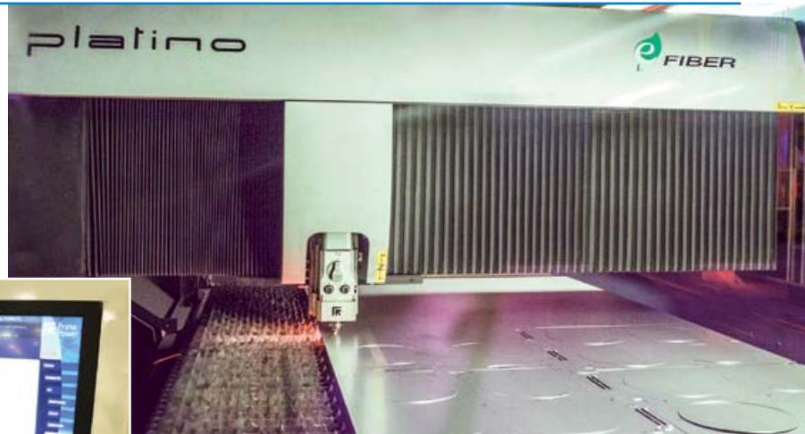
The Platino Fiber laser can be used to cut a wide range of materials. Fiber lasers are more effective than other laser sources for cutting highly-reflective materials (e.g. aluminum alloys, copper, brass). Platino Fiber cuts varied thicknesses, up to 20 mm of mild steel, with efficiency and quality. Productivity increases particularly with thin and medium-gauge sheet metal.
