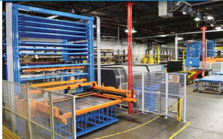
Prima Power's Compact 10-shelf TowerServer allows easy loading/unloading for blanks and processed sheets. It has an elevator for loading and unloading the pallets on and off the tower, and features single sheet separating, control systems, and sheet reference. The Platino Fiber is particularly suitable for 24/7 operation, often performed in unattended mode.
