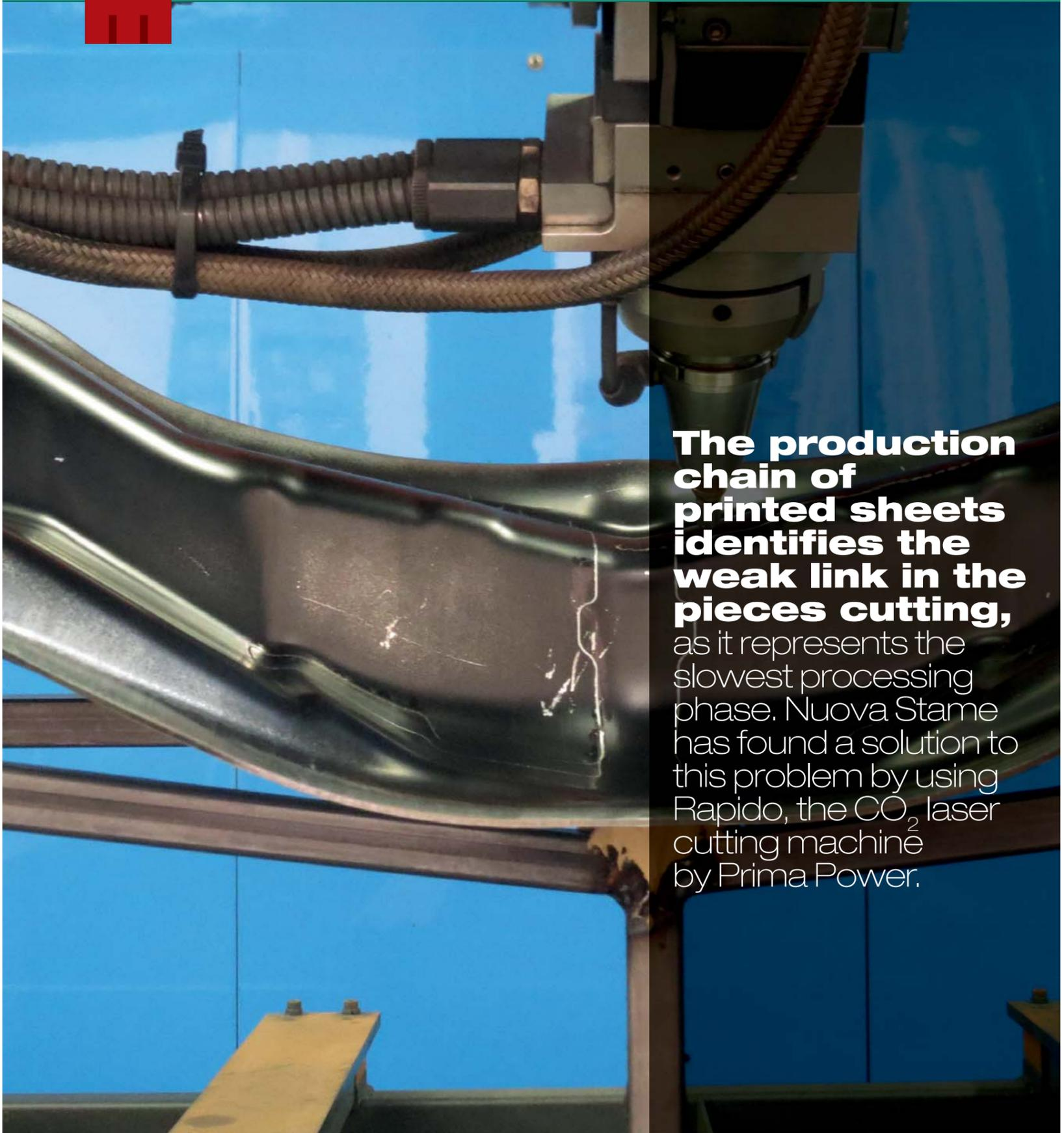
**The production chain of printed sheets identifies the weak link in the pieces cutting,** as it represents the slowest processing phase. Nuova Stame has found a solution to this problem by using Rapido, the CO<sub>2</sub> laser cutting machine by Prima Power.
