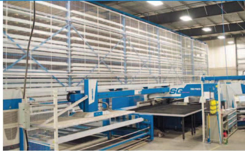
The Shear Genius increases material productivity through efficient and versatile nesting programs. The level of automation can be customized through Prima Power's flexible modular solutions for raw material storage, loading, unloading, sorting and stacking. These features can be added later as budgets allow and production demands increase.
