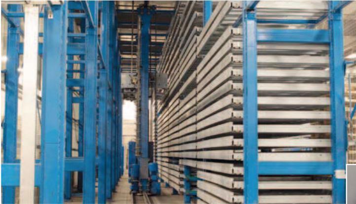
The Night Train Material Management System is an inventory and material transporting center. It provides a total solution for unmanned operation for sheet metal fabricators by automating system control, as well as material flow within the system. This includes supplying raw material and removing and storing work in process.
