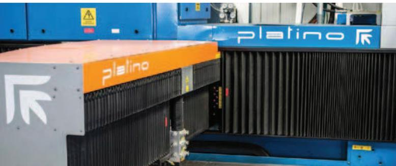
Carmeco chose the Prima Power Platino for the following reasons: cantilever arm, user-friendly software, one-piece stonecast construction, and flexible automation.
