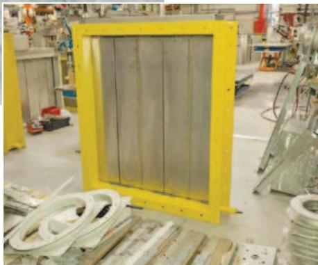
Fire damper manufactured by Halton Marine.
