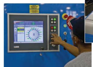
With the E5x by Prima Power, modern servo-electric punching productivity is available in a flexible and affordable package. It has been designed to offer versatile capacity made easy to utilize. Prima Power's new machine control and user interface software with touch screen panel ensure fast set up and convenient operation.
