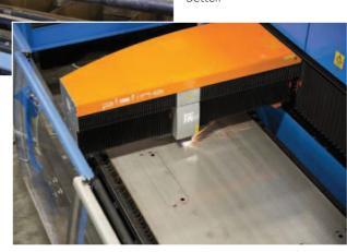
Offering a compact footprint along with a Cartesian Cantilever structure that provides three-sided access, Platino is a cost-effective machine that is easy to operate and quick to program.
