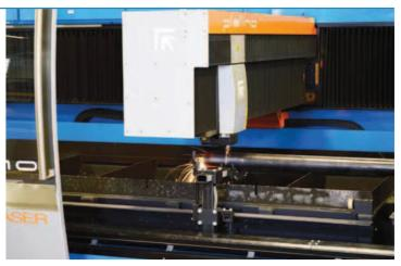
One of the Platinos' features that American Industrial Heat Transfer especially liked was the rotary axis option for tube cutting. With zero set-up time, the Platino can change from cutting sheet metal to processing of round, square, and rectangular tubes.
