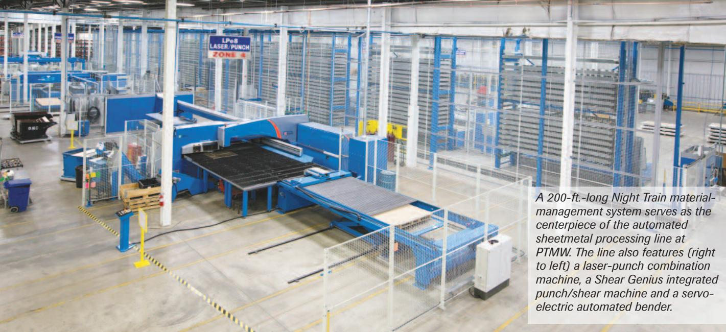
A 200-ft.-long Night Train material-management system serves as the centerpiece of the automated sheetmetal processing line at PTMW. The line also features (right to left) a laser-punch combination machine, a Shear Genius integrated punch/shear machine and a servo-electric automated bender.
