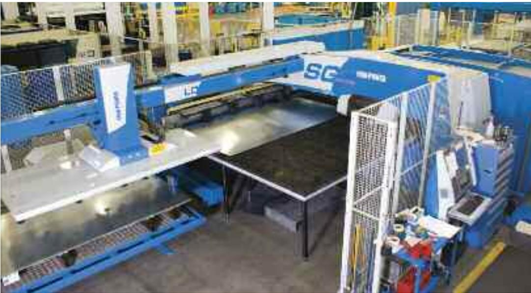
*With the integrated punch/right-angle shear combination concept, the objective is to provide one machine capable of transforming a full-sized sheet into punched parts. Sorting and stacking automation then moves the parts to secondary bending operations without being touched by human hands.*
