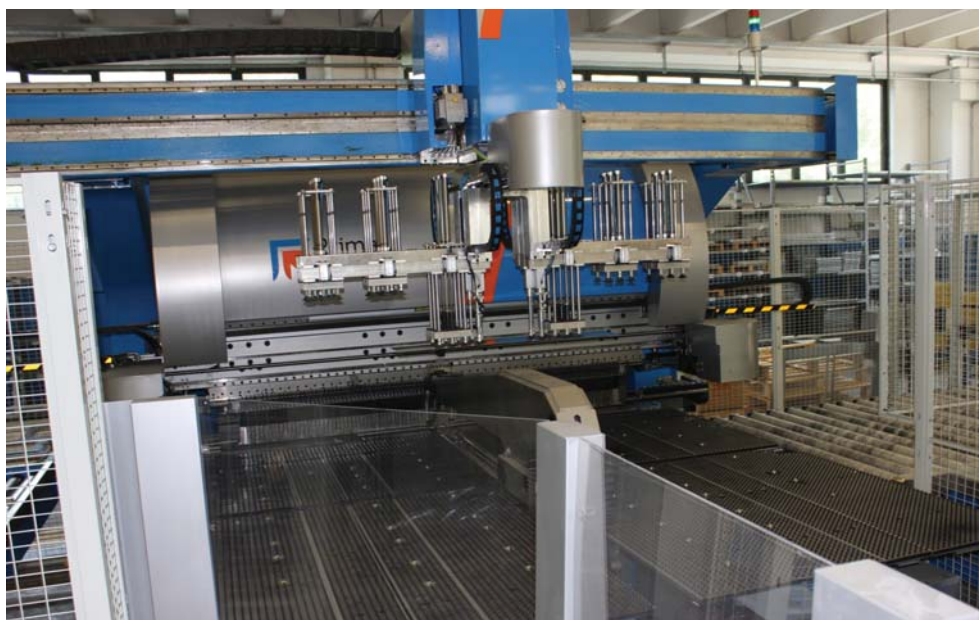
Fig.2 - The EBe 5 bending machine chosen by C.L.A. (Carpenteria Leggera Aerotecnica) is able to perform the bending lengths up to 2,650 mm.
