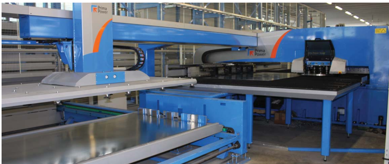
Fig.1 - View of the Prima Power Shear Genius SGe 6, integrated punching and shearing machine operating at the C.L.A. (Carpenteria Leggera Aerotecnica) plant.
