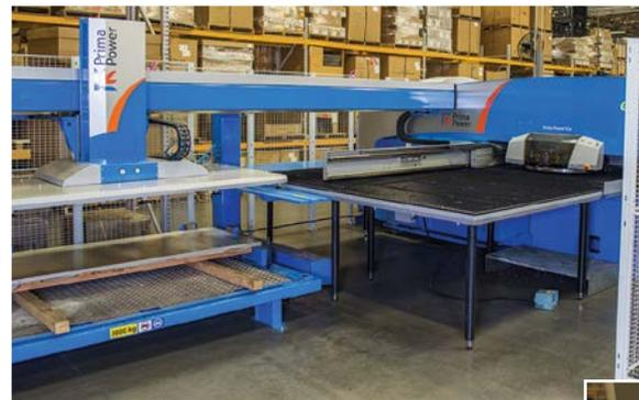
As loading, punching, forming & upforming, unloading, sorting, and stacking become automated, the result is a finished part with a dramatic reduction in scrap and manual labor while increasing productivity.
