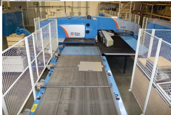
**Upward Forming System** – Prima Power's upward forming option provides more accurate forming and greater forming heights up to 16 mm (.63”). Another advantage is that all dies are at the same height and there are more high-forming dies in the turret, reducing risk of material damage and increasing machine uptime. “We use our upform station for producing louvers, lance, and forms on the new SGe cells,” adds Wise.
