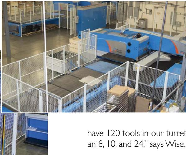
**Multi-Tool®** – Prima Power's Multi-Tool stations increase the number of tools available in a turret, thus reducing setup and increasing productivity. The Multi-Tool system allows multiple tools to be put in one station. Prima Power's Multi-Tool and the drop-in and indexable Multi-Tools from Prima Power's tooling partners offers 6, 8, 10, or 24 different punch/die combinations in only one station – a turret within a turret. “We
