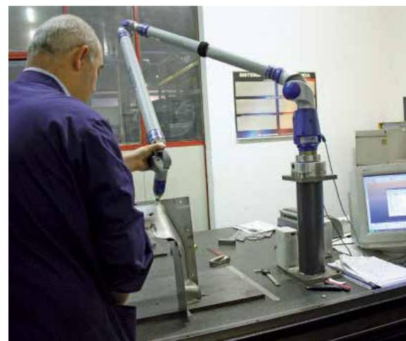
FaroCam2Lasersystemformeasurementandcontrol in use at the company IMPEA for examining the accuracy of the components produced. (Lasertec photo)
