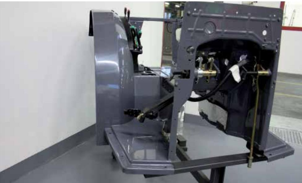
Vision of the front frame of a tractor with control foot switch. (Lasertec photo)
