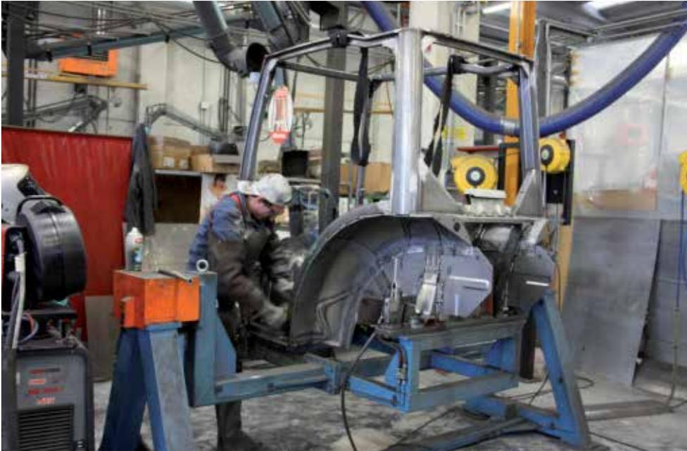
Grinding of components of a tractor cabin. (Lasertec photo)
