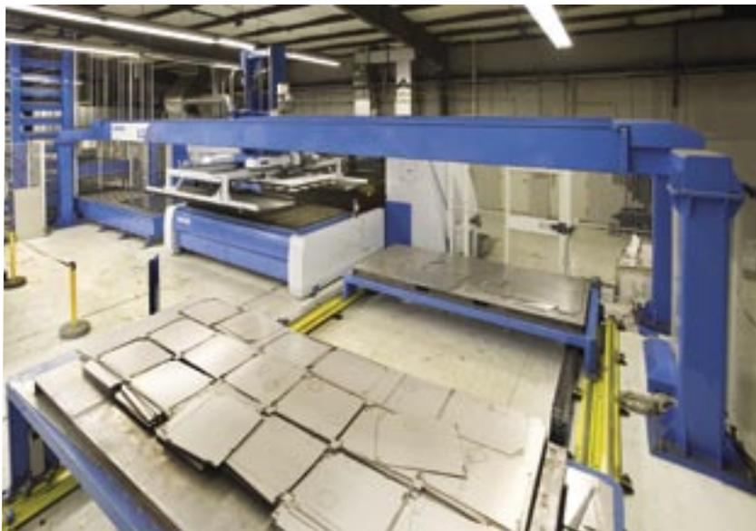
**Great Lakes Manufacturing uses technology, like the new Finn-Power laser and automated materials handling equipment, to differentiate itself from competitors.**
