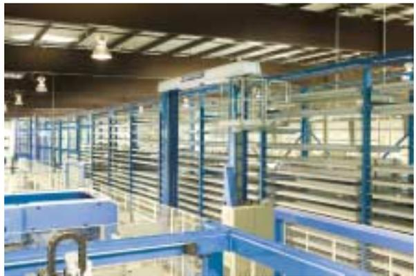
**The Night Train doesn't stop and now stretches almost the entire length of the Advanced Automation Center to inventory and deliver sheetmetal material to the four Finn-Power machines.**
