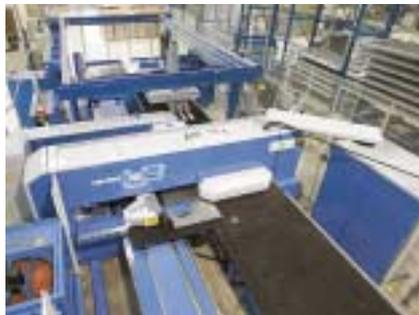
Laser Brilliance combines a 3.5kW laser with Finn-Power's hydraulic 30-ton station, 30-ton turret punch press and linear drive technology for extremely fast and accurate positioning.
