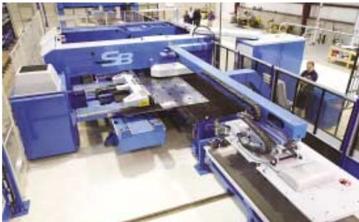
The Shear Brilliance FMC punch/shear machine combines processes into one lean manufacturing operation.
