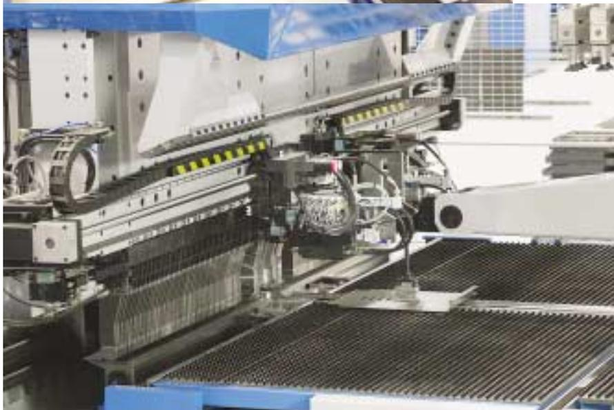
The Express Bender automates complex bending and the operations cycle from loading full size sheet to unloading bent parts.
