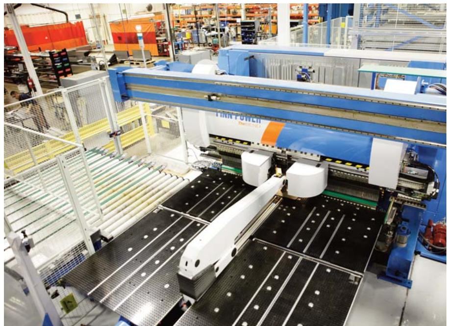
FIGURE 4 The automated bender has changed the way Siemens engineers design metal parts. In fact, if a part is larger than 6 in., it is reviewed to see if it can be redesigned to take advantage of the automation.
