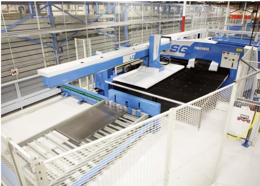
**FIGURE 1** Avoiding or minimizing setup of any kind is an important part of maintaining high levels of productivity. To maximize throughput on its new Shear Genius punch/right-angle shear combination machine, Siemens Industry Automation maintains a fixed set of tooling on the machine and feeds as many parts as possible through it, taking full advantage of the system's automated material handling.
