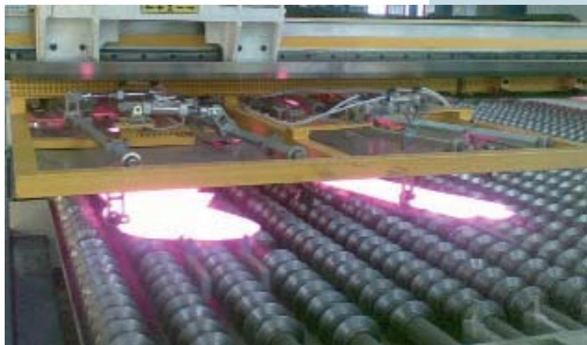
FIG[03] Blanked components inside a furnace that brings them to a temperature of 930 °C.
