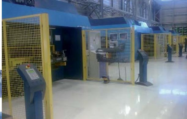
FIG|05| Four Rapido laser systems to trim hot moulded parts. Each unit is powered by a CO2 source with 4 kW power.
