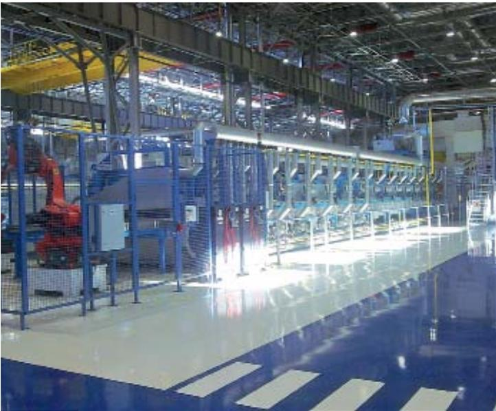
FIG[02] One of 5 sheet heating furnace lines with, on the right, the previously blanked components hot moulding press.
