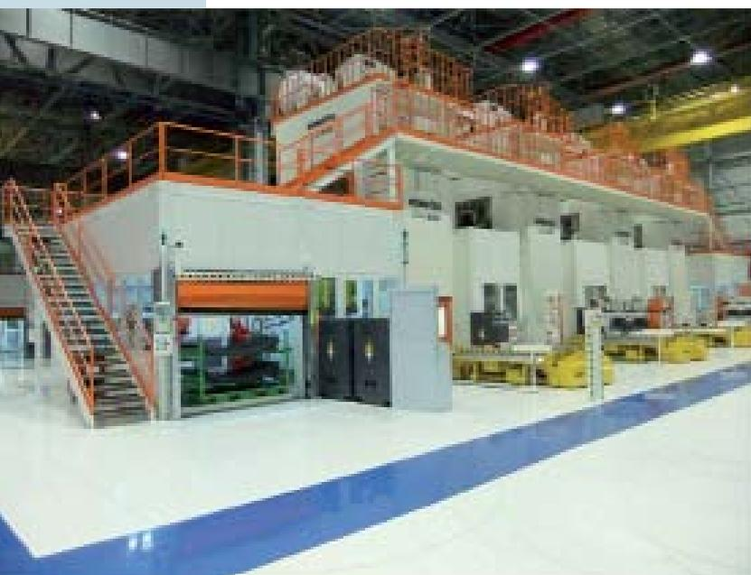
FIG|04| Mechanical presses line for automatic trimming and perforation of hot moulded parts.
