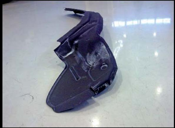
FIG|07| Examples of windscreen upright bars before (a, b) and after (c, d) laser trimming using the Rapido systems in the Cassino plant dedicated to bodywork, hot moulded parts
