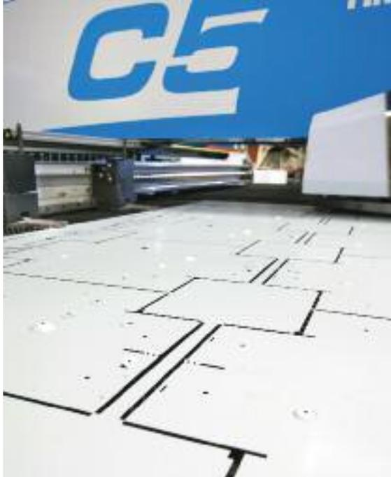
Software allows part nesting on a full sheet, reducing material usage and the need to pay premium prices on customized blanks for the turret punch press.
