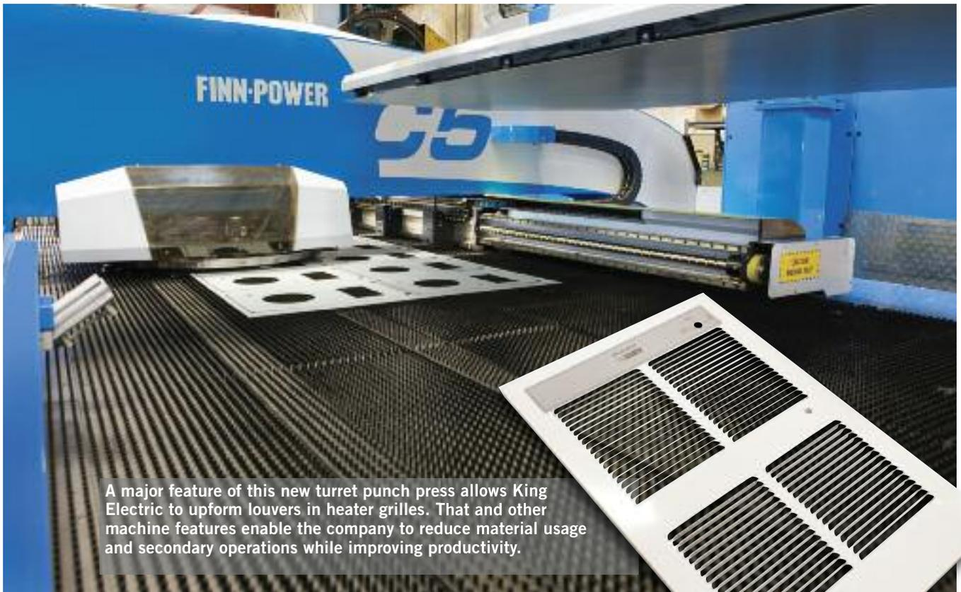
A major feature of this new turret punch press allows King Electric to upform louvers in heater grilles. That and other machine features enable the company to reduce material usage and secondary operations while improving productivity.
