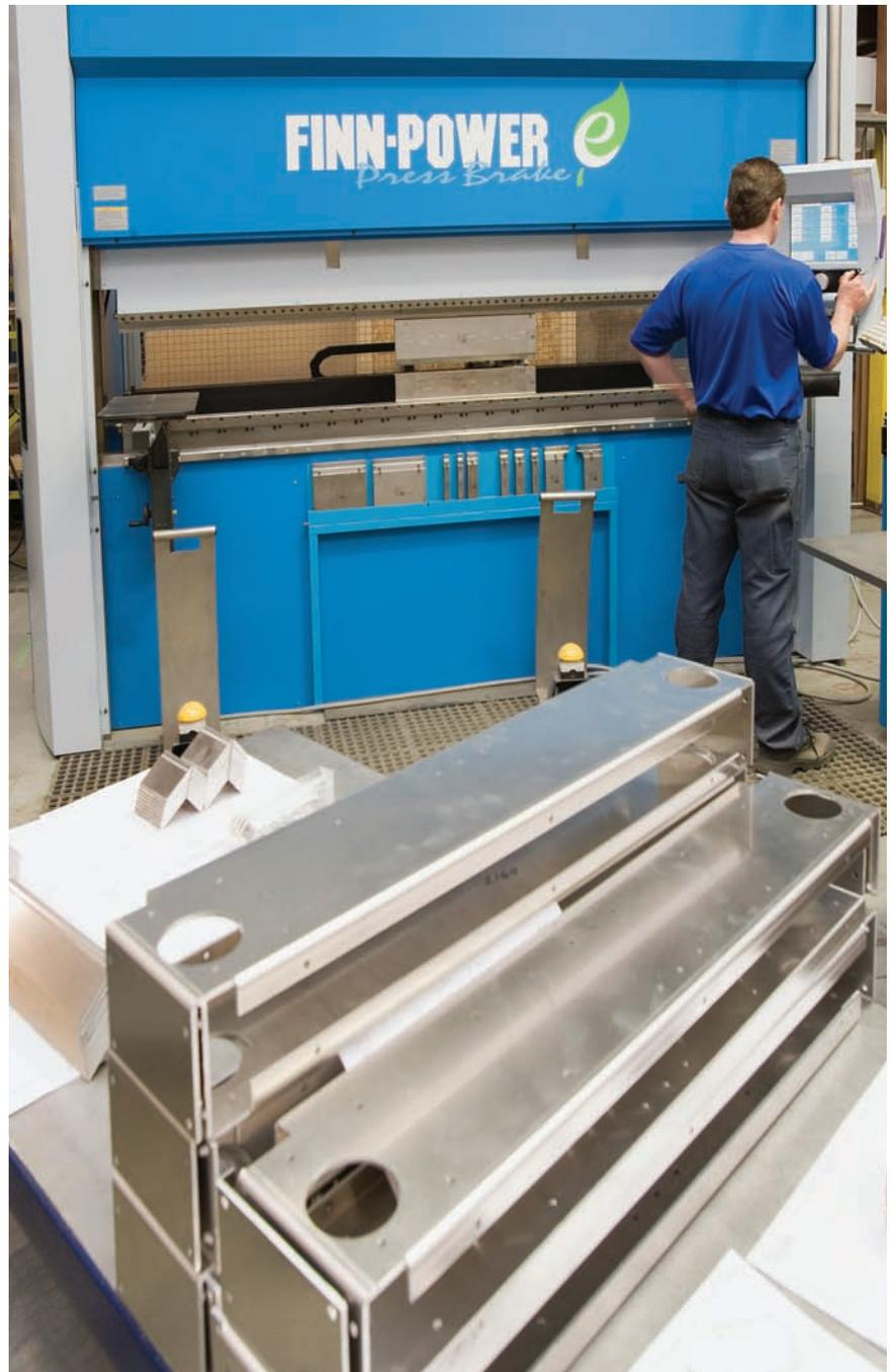
A new servo-electric press brake operating at Laicor Fixtures boasts a patented drive, based on the pulley principle, which evenly distributes forces in the top beam. The result: optimum accuracy, increased productivity and decreased energy consumption, with minimal maintenance requirements, claim Laicor officials.
