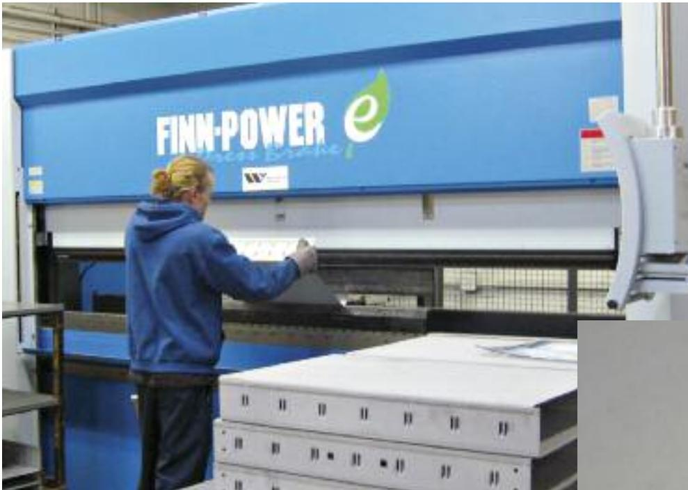
The firm equips its servo-electric press brake with a tool that hems and bends drawers in one setup, a big time saver compared to its previous hydraulic press brake that required separate hem and bend tools. Note (below) the series of bridge lances formed on the drawers—the C5 turret press upforms these features (a patent-pending drawer design) to locate drawer dividers.
