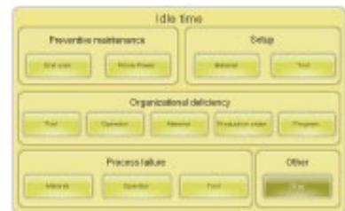
Idle times can be defined by the user to describe the reason why the machine was idle, for example: lunch or coffee break, tooling change, stacking area clearance etc. Fault error messages are recorded to identify what alarms occurred during this time.
