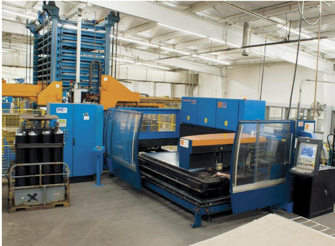
*In order to expand its laser cutting capabilities, Pulverman purchased a Prima Platino 2D laser system with a 10-shelf TowerServer in 2004. The Platino is equipped with lasers developed and produced at Prima Industrie in laser powers ranging from 3000 to 5000W. The laser cuts a broad range of materials and thicknesses with speed and precision without the need for manual adjustments.*
