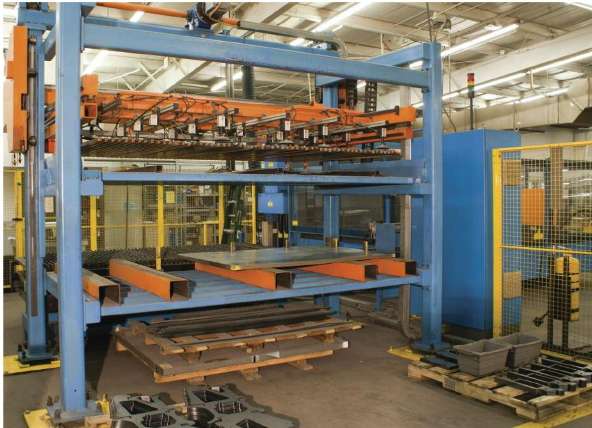
*In 2006, Pulverman purchased a second Platino laser with a load/unload. According to Yermal, the flexibility of the load/unload gives Pulverman the ease of loading and unloading sheets, just like on the large tower. All the operator needs to do is touch a few buttons to unload a scrap sheet and load a new sheet. With the load/unload, the company can just load the material that it is running at that moment.*
