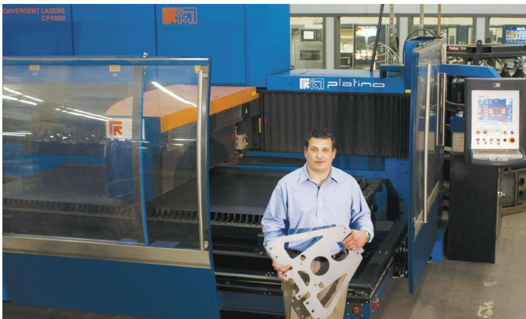
*According to Ken Yermal, engineer, while lights out automation is not a major part of Pulverman's current production, the Prima Platino lasers have helped the company trim labor costs. With two people, the company is able to run all three Platino lasers efficiently, and have parts that are already out of the skeleton and ready to move to the next operation. In most cases, no deburring operations are needed.*
