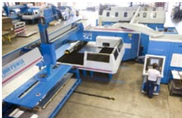
**On average, Shear Genius reduces total manufacturing time by 60 percent and saves one blank sheet out of every 10. With the Shear Genius, SPM estimates it has reduced material costs by 15 to 20 percent**
