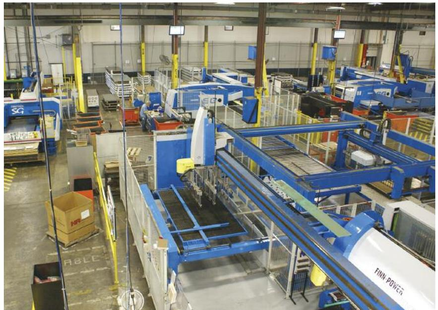
*Through the years, the Emerson Columbus, OH facility has added new generations of Shear Genius equipment to its fabrication arsenal. Today, it has a total of five Shear Genius cells and one Laser Punch cell.*
