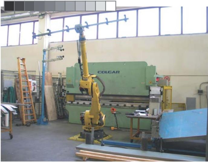
Colgar Bending machine, with a robotised plate metal handling system, installed at MBM premises
