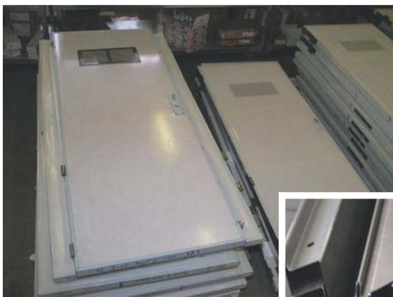
Examples of doors with relative frames produced by MBM. Note the precise bending work on the metal sheet previously cut with the laser
