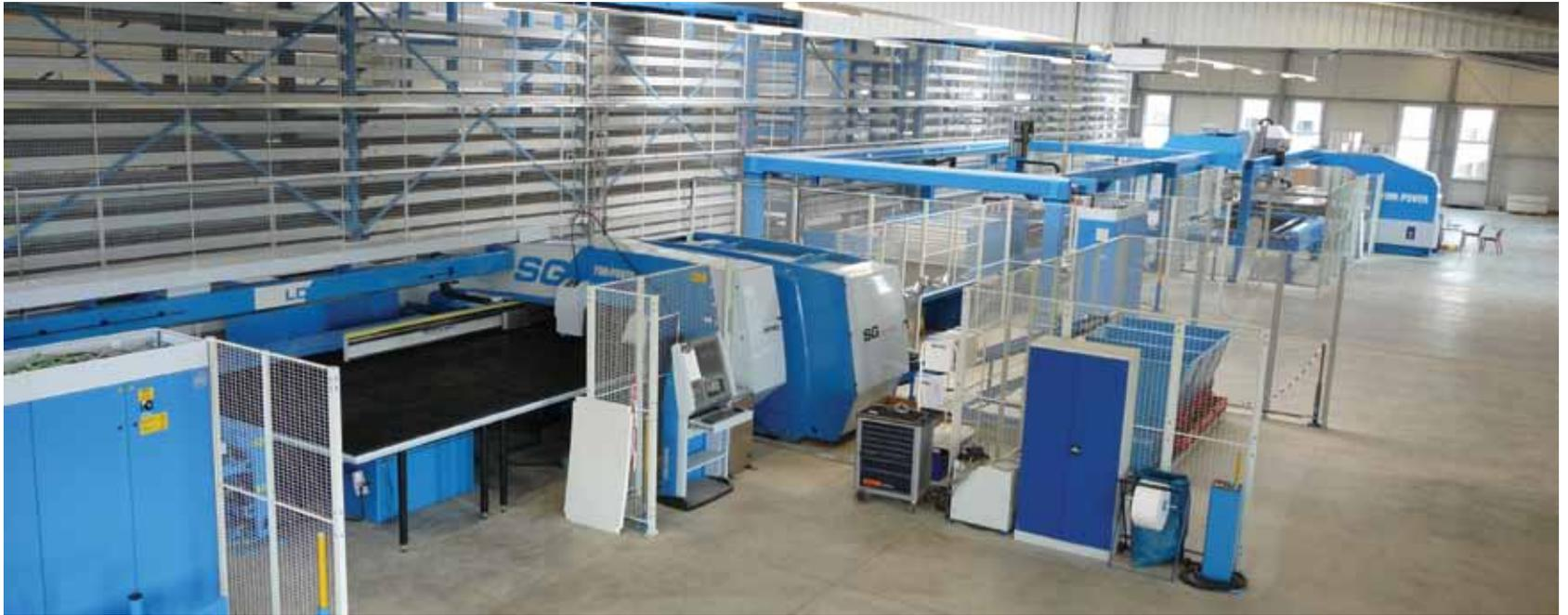
A visit to HT Labor+Hospitaltechnik AG, Heideck, Germany, gave us the opportunity to observe the operations of a Finn-Power (now Prima Power) automated fabrication and bending line for continuous processing of steel and stainless steel sheets, which are used to make modular walls, ceilings and doors for hospitals and bio-medical research laboratories.
