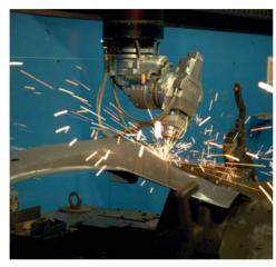
For typical thicknesses of the parts considered, ranging from 1 to 2 mm, today the work advancement speed obtained is over 20 metres per minute, with a process duration of about 30 seconds per part.
