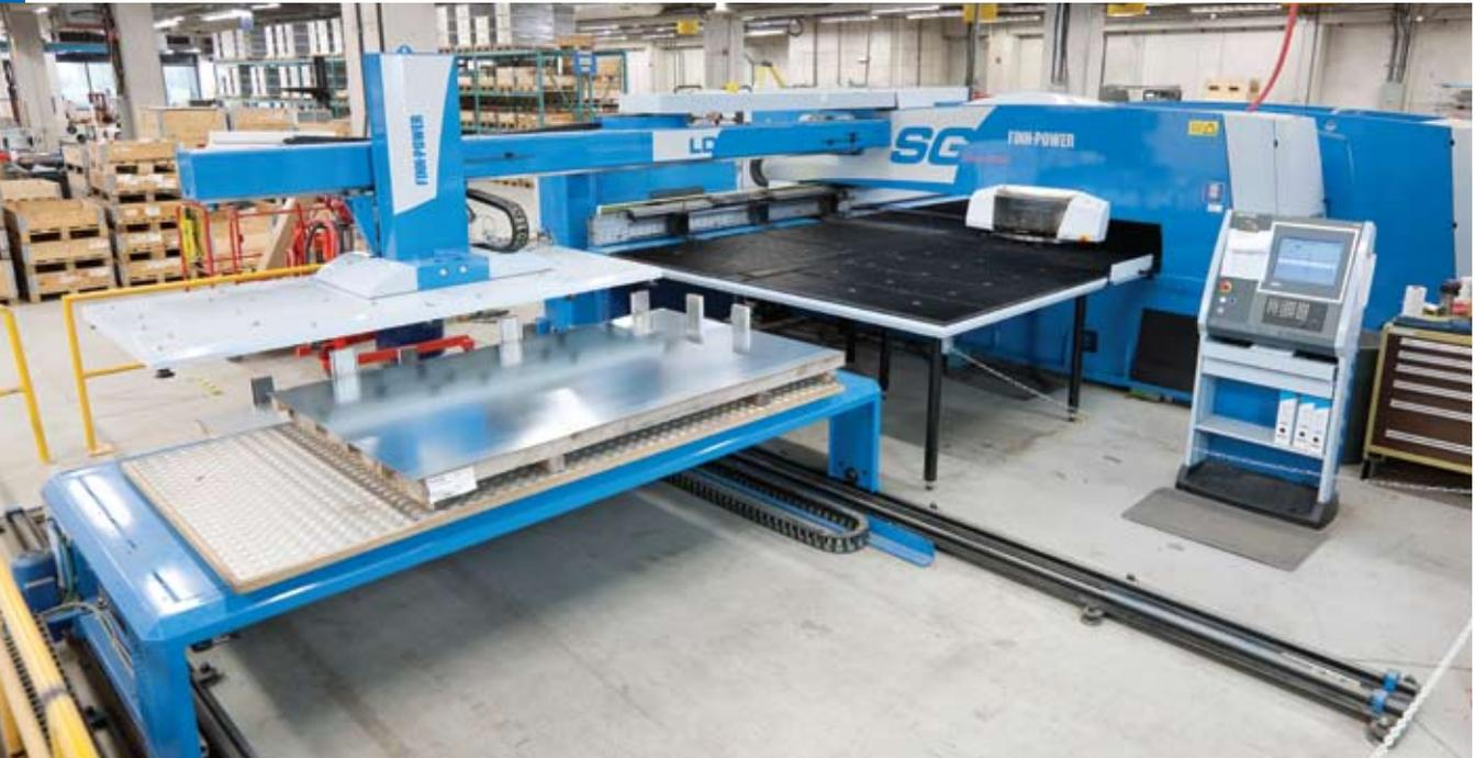
Because the loading, punching, and shearing of parts is automated, there is a reduction in scrap and manual labor.
