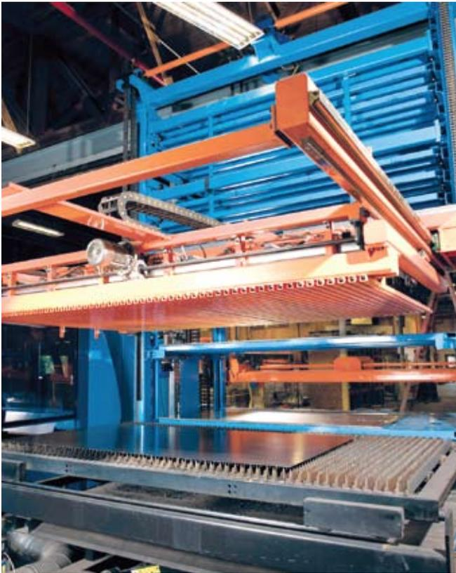
The Prima Sincrono laser with the TowerServer in the background. The system is capable of Lights Out operation, a feature that appealed to Rob Marelli.
