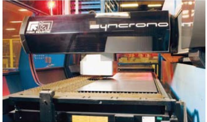
Seconn's latest acquisition is the Prima Sincrono laser with TowerServer, an automated work handling system. Marelli liked the lights out capability of the laser machine.
