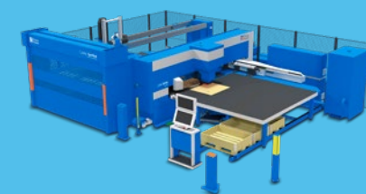
Combined machines with punch and laser
