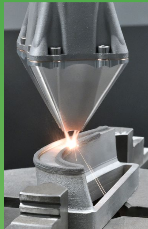
Turbine vanes are repaired with Prima Additive technology
