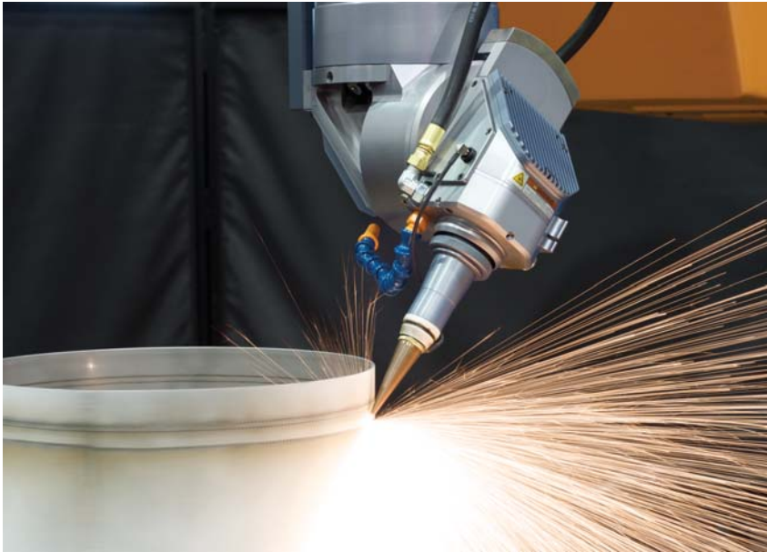
LASERDYNE BEAM DIRECTOR DRILLING A 3D AEROSPACE COMPONENT
