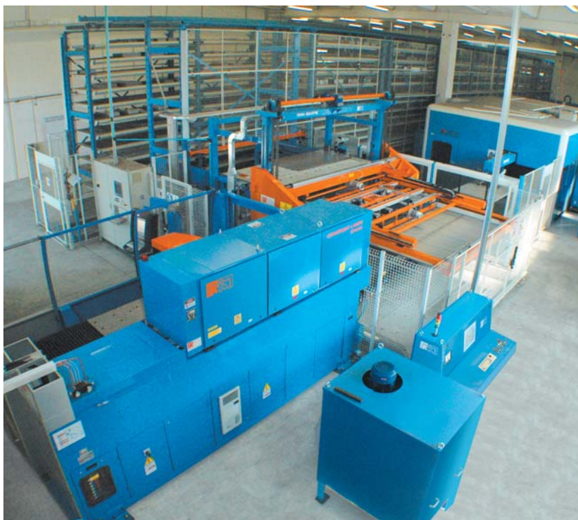
FLEXIBLE MANUFACTURING SYSTEM FOR LASER CUTTING, PUNCHING AND SHEARING INSTALLED IN ITALY
