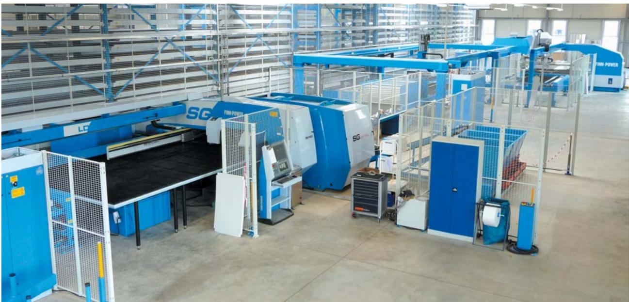
FLEXIBLE MANUFACTURING SYSTEM FOR PUNCHING-SHEARING-BENDING INSTALLED IN GERMANY
