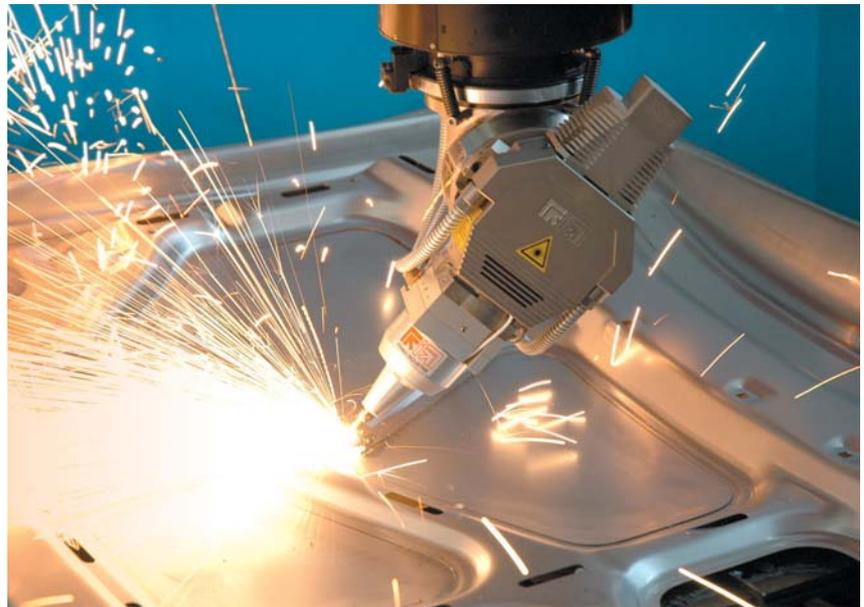
3D LASER HEAD CUTTING AN AUTOMOTIVE COMPONENT
