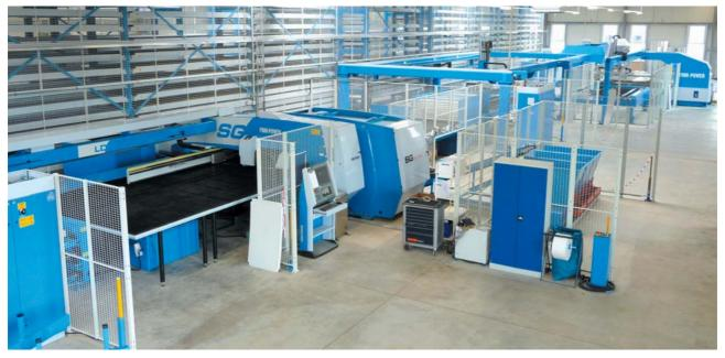
FLEXIBLE MANUFACTURING SYSTEM FOR PUNCHING-SHEARING-BENDING INSTALLED IN GERMANY
