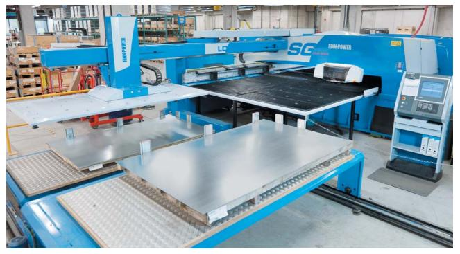
INTEGRATED PUNCHING-SHEARING CELL SHEAR GENIUS
