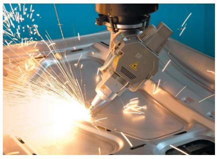
3D LASER HEAD CUTTING AN AUTOMOTIVE COMPONENT
